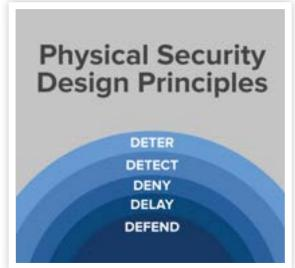
The deterrence layer is the visible barriers including anti-climb, anti-cut fencing, high-security gates, surveillance cameras, signage, watch guards, and more. The detection layer is the alarm function of these perimeter solutions and can be enhanced with additional non-visible monitoring solutions like drone detection, buried sensors, embedded sensors, hidden cameras, radar, lidar, or other detection systems.
